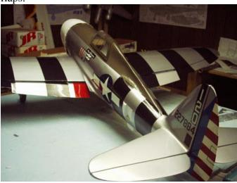
He plans to power this plane with a Super Tigre G-75 engine and use a JR6103 with standard 537 servos. This is his first attempt at a scale model and he has been working on it since last August. He states that it is near completion and will be flying before long.
