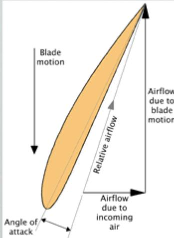
*The relative angle of attack of the airflow to the propeller blade depends on the rotational speed of the blade, and the speed of the incoming air flow.*
