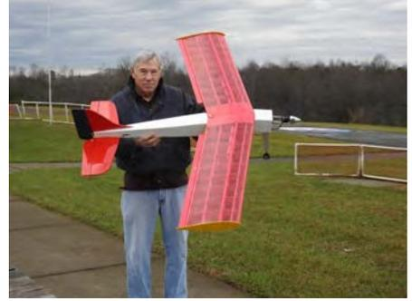
Bob Cunningham designed pattern trainer, originally for 40 size engines but converted to electric. Cunningham designed it at the behest of a man named Hooker, hence the name of the plane. The plane is receiver ready and includes a 5000mAh 4S battery, it is best described as a Stick with a swept wing. Weight is 4 pounds 10 ounces and it has a brand new Cobra motor. It is an easy plane to land and is either gentle to fly or violent if you like 3D flying depending on your setup.
